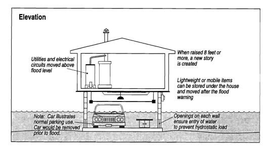
Cost is an important factor to consider in elevating structures. Lighter wood frame buildings are easier and cheaper to raise than masonry buildings. Masonry buildings not only are more expensive to raise, but are susceptible to cracks. If homeowners opt for elevation of the building, they must not then place contents or materials susceptible to flood damage on the new lower level.
