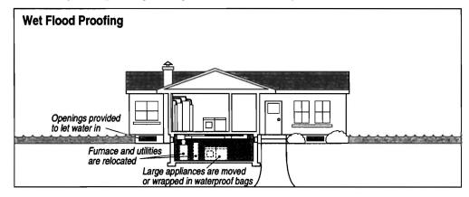
Wet flood proofing is generally appropriate in cases where an area is available above flood levels to which damageable items can be relocated or temporarily stored. This approach is also appropriate for structures with basements and where other flood proofing measures will not be effective.
